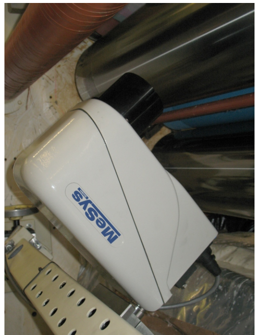
Thin coating measurement on coating roller (lamination line)
